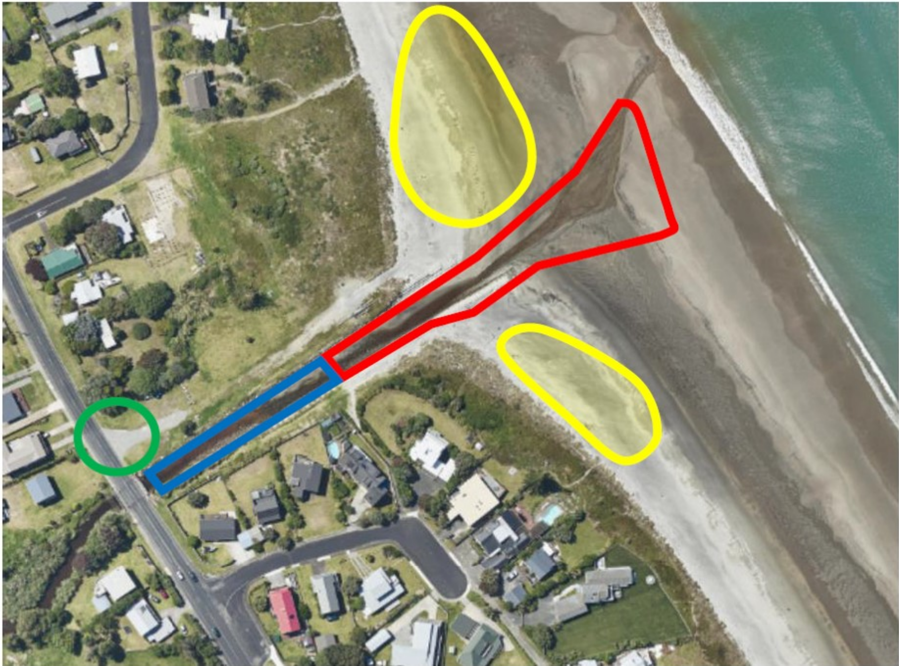
Figure 8. Three Mile Creek proposed excavation (blue: Zone A and red: Zone B) and deposition areas (yellow) and access point (green) (source: Bay of Plenty Maps)
