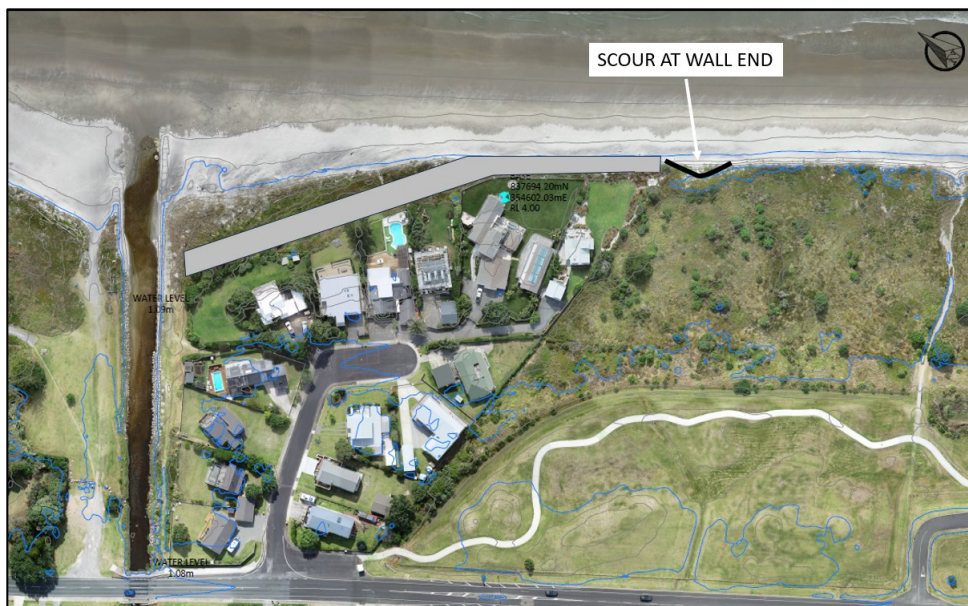
Figure 23: Potential scour at southern wall end
