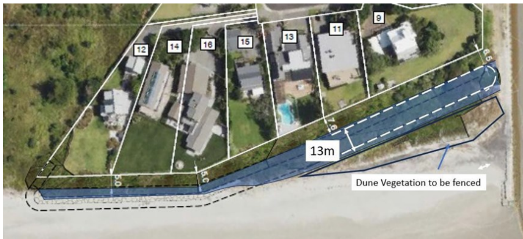
Figure 21: Indicative location of vegetation removal (blue) and northern dune vegetation to be protected (Source: Construction Methodology).
