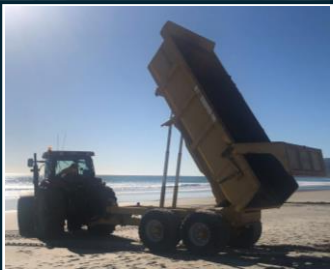
PNEUMATIC TRACTOR/TIPULATOR DUMPS ROCKS FROM RESERVE DOWN CIRCA 4m INTO CREEK BED
