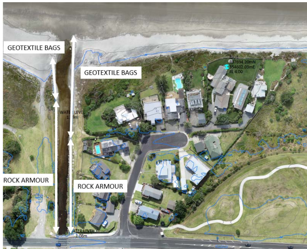
Figure 3.4a: Armoring to 3 Mile Creek
