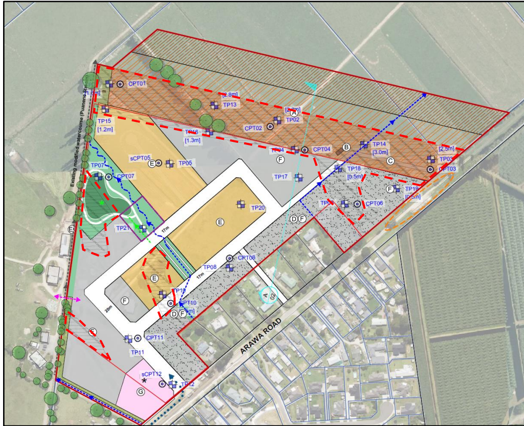
Figure 1: Image overlapping CMW test locations and peat soil observations against the spatial provisions of the Structure Plan. The OLFP between the looped road has been located as shown to ensure separation of upstream overland stormwater and floodwater flows from the stormwater treatment wetland.
