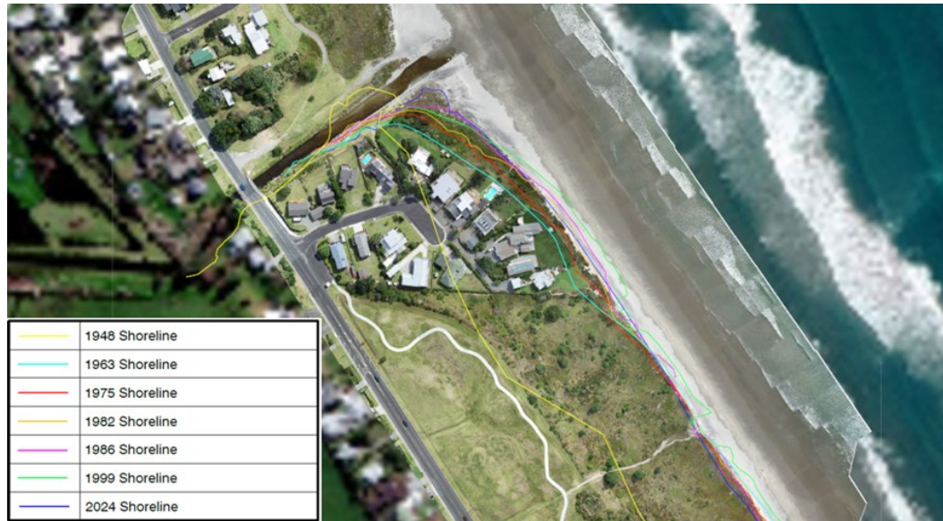
Historic coastlines overlaid on 2024 aerial (Figure 3.5a from the Coastal Processes Assessment, Davis Coastal Consultants, October 2024).
