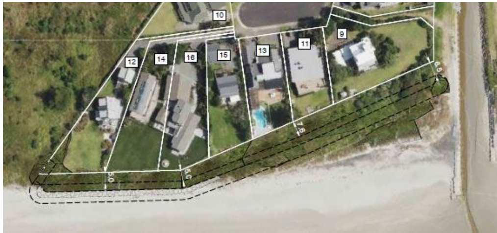
Layout of rock wall (Figure 2.0a from the Construction Methodology Statement, Davis Coastal Consultants, October 2024; page 7).
