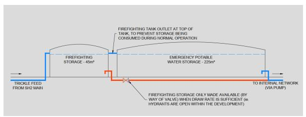
Figure 17: Diagrammatic representation of a potential conceptual reservoir arrangement at the site entrance.
