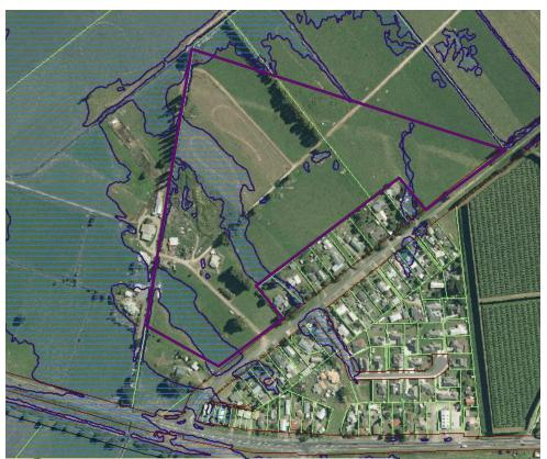
Figure 3: Flood mapping on site (from WBOPDC Maps)
