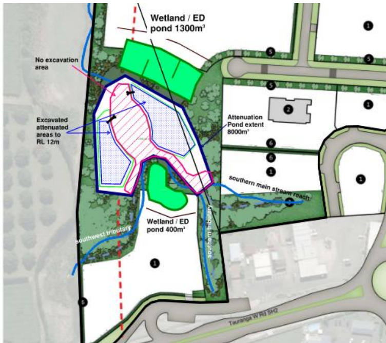
Figure 1 General Stormwater Layout.
