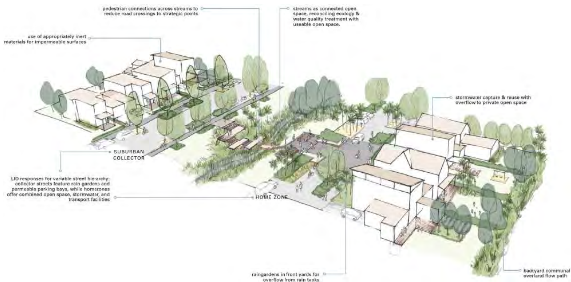
Figure 7-1: Example of suburban development that incorporates a water sensitive design approach (Lewis et al., 2013)
